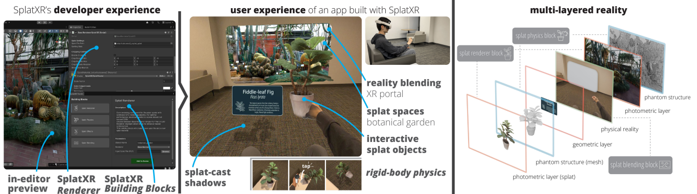
Figure 1: Left: A developer composes an XR app using our SPLATXR toolkit in Unity. Mid: The resulting app can be deployed to a standalone Meta Quest 3 or Apple Vision Pro headset, featuring several toolkit capabilities for a rich, interactive user experience. Right: The toolkit leverages a set of custom SPLATXR representations.
